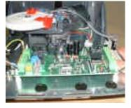
11. Using flat blade screwdriver, press barb on PCB spacer to compress it, at the same time lift the PCB gently up to remove it from spacers (x4.)
