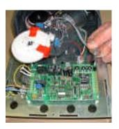
8. Remove limit switch connector.
