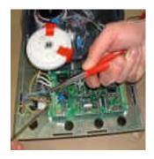
9. Carefully noting position of remaining wires – press orange tabs down and remove wiring from terminal blocks. (There is a wiring diagram inside lid of unit.)
