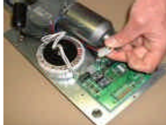
8. Remove wire from motor.
