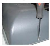
1. Unscrew retaining screw in Operator cover and remove.
