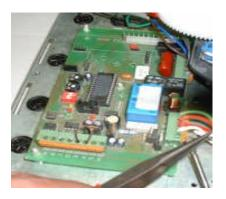
5. Push back orange retaining clip and remove all wires from both terminal blocks.
