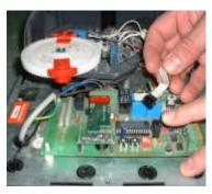
2. Pull back black retaining clip and remove limit switch cable.
